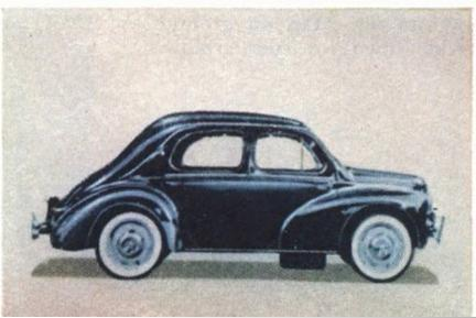
**40** Renault 4CV sedan with 83-inch wheelbase, 28-hp four-cylinder, water-cooled engine, \$1,345
