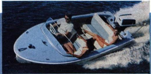
The Playmate 14' runabout. Has lapline hull, sealed double bottom-flat floor. Foam seats. Rear seat reverses for water ski observation and trolling. Complete \$745.\*
